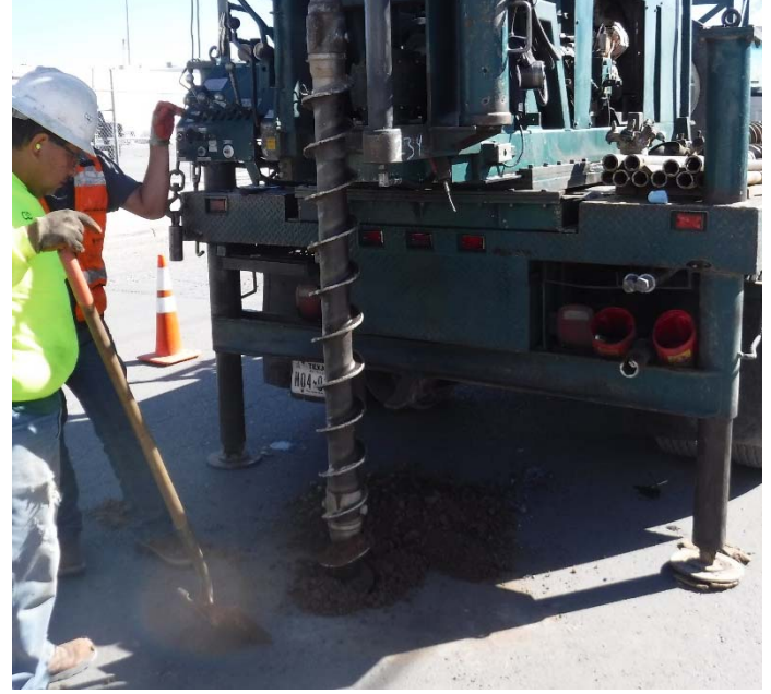
PHOTO NO. 14: General view of drilling activities at exploration soil boring 2B-9 location.
